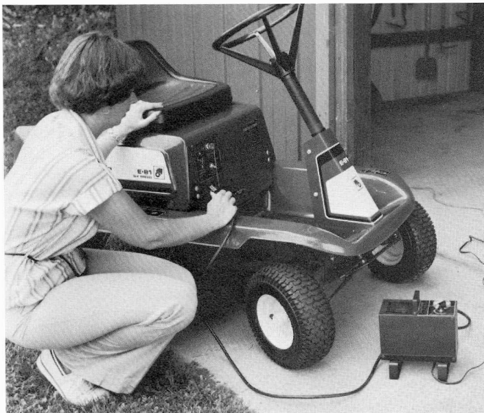
A battery charger included with the E-81 will recharge the unit overnight.
