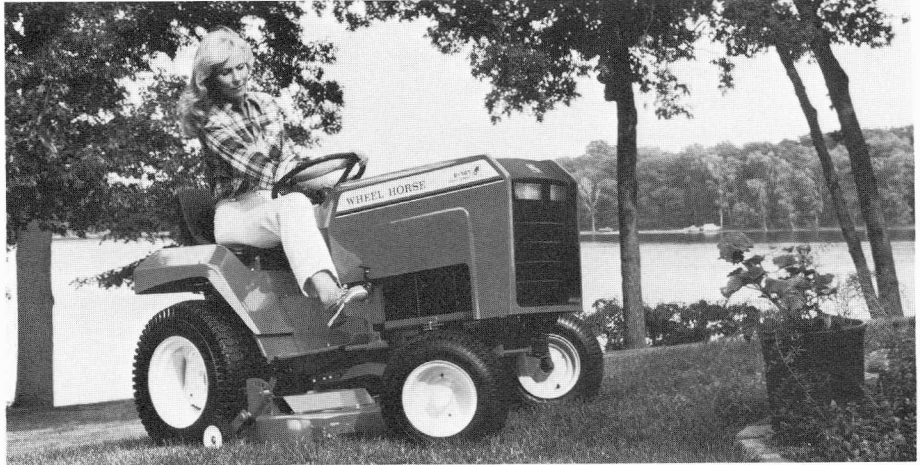
The Wheel Horse E-141 lawn tractor combines the rugged components of other Wheel Horse tractors with quiet, economical battery power.
